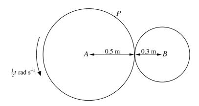
Two coplanar discs, of radii 0.5 m and 0.3 m, rotate about their centres A and B respectively, where AB = 0.8 m. At time t seconds the angular speed of the larger disc is  $\frac{1}{2}t$  rad s<sup>-1</sup> (see diagram). There is no slipping at the point of contact. For the instant when t = 2, find
